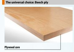
Worktop for **general requirements.** Made of peeled beech veneer, with multiple cross layers, glued, non-warping, and waterproof. The edges are smoothed, the surface is sanded and sealed with clear UV varnish.
