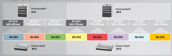
The **coloured areas** for the individual products indicate the relevant **inside drawer dimensions** in G units. In group 95 – GridLine accessories – you can use the colour scheme to find the most suitable dividing material for your drawers in a quick and uncomplicated manner. Colour of the drawer = colour of the dividing material.
