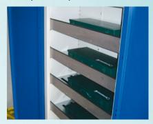
Simple protection against tools falling out, for instance when a cupboard is opened.
