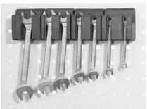
Clear storage of the spanners. Spanner size is clearly visible through the opening.
