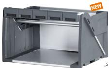
Cable reel carrier made of plastic with aluminium axle **dia. 12 mm** and wire holder dia. 6 mm. Wire holder with cable guides, prevents unbraked unrolling of the cable. The depth of the wire holder can be adjusted. Aluminium axle can be mounted in 3 positions so that rolls with dia. 100, 200 and 300 mm can be attached.
