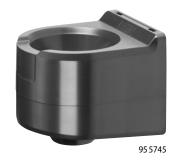
To take compressed air guns with or without connection hose. 3 storage options: Mounting at the coupling  $(diameter\ of\ the\ stepped\ hole\ 26\ and\ 23\ mm,\ suitable\ for\ hose\ diameter\ up\ to\ 16\ mm),\ mounting\ at\ the\ male$ coupling (sleeve diameter 13 mm) or hanging from the trigger.
